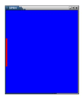
In here, heat is apply to the middle left corner of the plate. (red area represent the heat, and the blue area is the plate).
