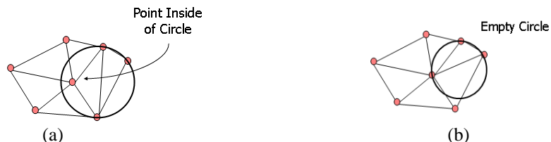
Figure 3: Examples of triangulations in 2D. (a) not a Delaunay triangulation, (b) Delaunay triangulation.
